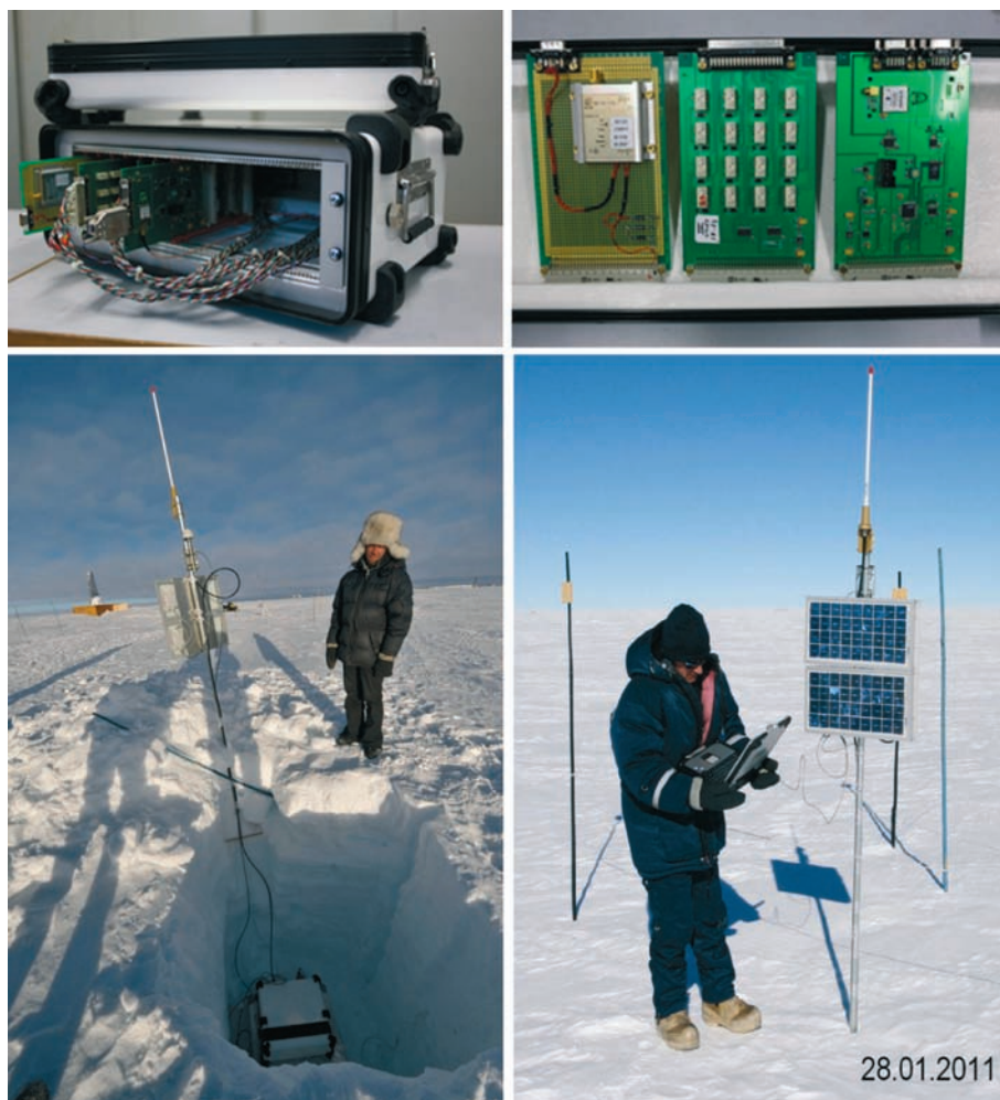
Fig. 1. TAUTO recording system and its setting in the field.
