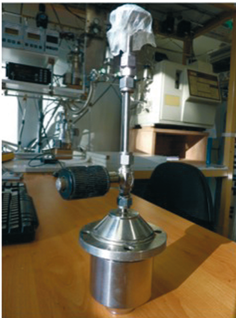
Fig. 4. Dry extraction method used for CO 2 measurements. The picture shows a closed stainless container with metallic balls inside, used at LGGE for pulverising ice samples under vacuum and extracting the gas for CO 2 measurements
